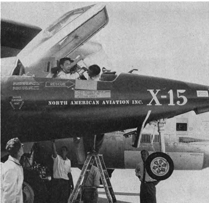
**FINAL CHECK** is made before Crossfield is locked in under the wing of B-52 that launches the X-15. The over-all shape of the stubby, fifty-foot manned vehicle is result of 4,000 hours of wind-tunnel runs of model planes.
