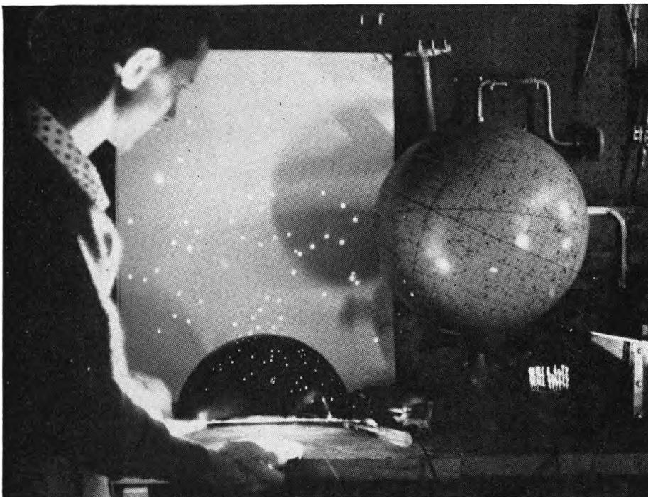
**SEVENTEEN-YEAR-OLD ASTRONOMER** *Charles Jones, Jr., has been studying the heavens since he was eight, recently built this planetarium, in which lights inside the half sphere cast moving star patterns on a small screen. He is currently working on a much larger model that will project constellations 30 feet to a dome.*
